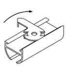
Distance between brackets max 1000 mm. Extra holders/brackets are recommended where the curtain is parked, when not in use. Recommended distance if holders are used together with brackets:
