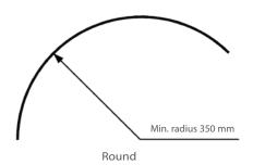
The track can be bent into complicated shapes, even in combinations of angle and round bending. Important! Front and back need to be specified on drawing/order. Contact Customer Service for more detailed information.
