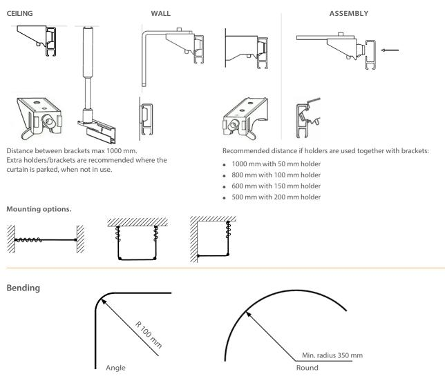
The track can be bent into complicated shapes, even in combinations of angle and round bending. Important! Front and back need to be specified on drawing/order. Contact Customer Service for more detailed information.
