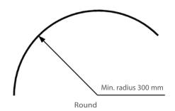
The track can be bent into complicated shapes, even in combinations of angle and round bending. Contact Customer Service for more detailed information.
