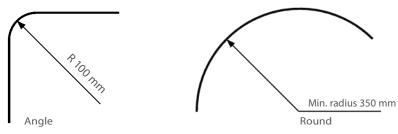
The track can be bent into complicated shapes, even in combinations of angle and round bending. Important! Front and back need to be specified on drawing/order. Contact Customer Service for more detailed information.
