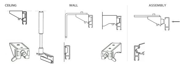
Distance between brackets max 1000 mm. Extra holders/brackets are recommended where the curtain is parked, when not in use. Recommended distance if holders are used together with brackets:
